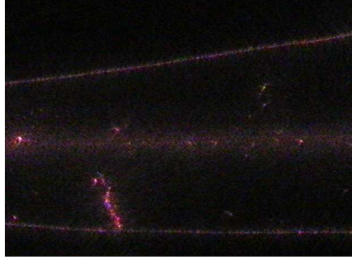
FIGURE 4.3: Image of prism coupled guided light by the Er:Ta 2 O 5 waveguides
