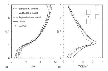
Figure 13. Vertical profiles of streamwise velocity and turbulence kinetic energy.
