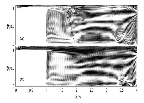
Figure 8. Mean velocity vectors in the x-z plane at  $y/Z_H=1.5$ . (a): LES32, fine mesh; (b): DNS64 (every two vectors plotted). Note that for the two cases different plotting routines were used, having small differences in arrow geometry.
