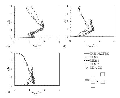
Figure 5. Vertical profiles of turbulence intensities in front of cube.
