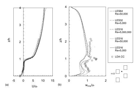
Figure 9. Vertical profiles of turbulence statistics at various Reynolds numbers. (a): streamwise mean velocity; (b): turbulence intensity.
