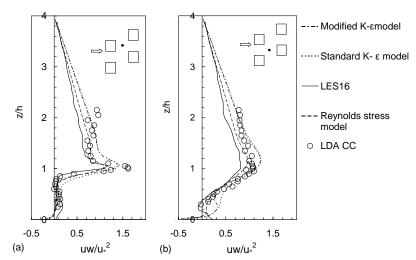
Figure 15. Vertical profiles of Reynolds shear stress behind and in front of the cube.
