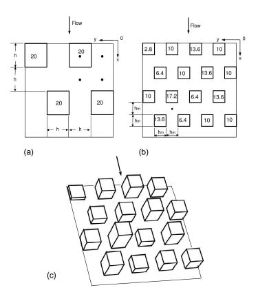
Figure 1. (a): schematic plan view of the domain for staggered cube arrays (case designated C20S); (b): schematic plan view of one unit of the domain for staggered random arrays, which consists of  $2(\text{streamwise}) \times 2(\text{lateral})$  units (designated RM10S). Dimensions in mm, with element heights indicated; (c): perspective view of one repeating unit of RM10S.
