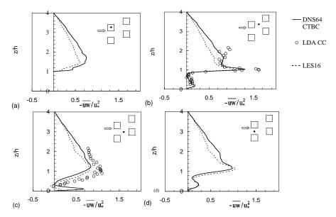
Figure 7. Vertical profiles of Reynolds shear stress at four horizontal positions. (a)over cube, (b)behind cube, (c)in front of cube, (d) in gap.
