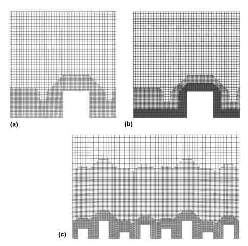
Figure 2. (a): mesh with finest resolution h/32 for C20S (LES32) at y=0.5h; (b): mesh with finest resolution h/64 for C20S (LES64) at y=0.5h; (c): mesh with finest resolution h/16 for RM10S at x=5 $h_m$ .
