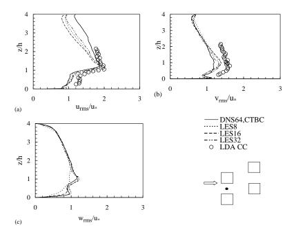
Figure 6. Vertical profiles of turbulence intensities in gap.
