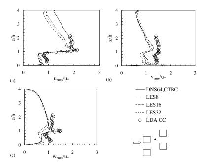
Figure 4. Vertical profiles of turbulence intensities behind cube.
