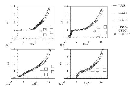
Figure 3. Vertical profiles of streamwise mean velocity at four horizontal positions. (a): over cube; (b): behind cube; (c): in front of cube; (d): in gap.
