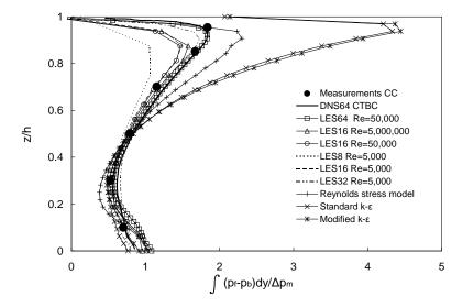
Figure 11. Vertical profiles of laterally-integrated pressure difference between front and back faces of the cube.
