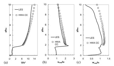
Figure 12. Vertical profiles of streamwise velocity and turbulence intensities behind 17.2mm obstacle, RM10S.
