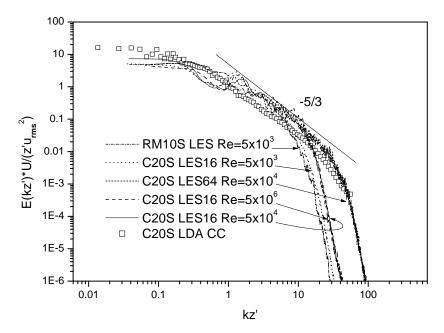
Figure 10. Spectra of the axial turbulence component, plotted in inner-layer scaling.
