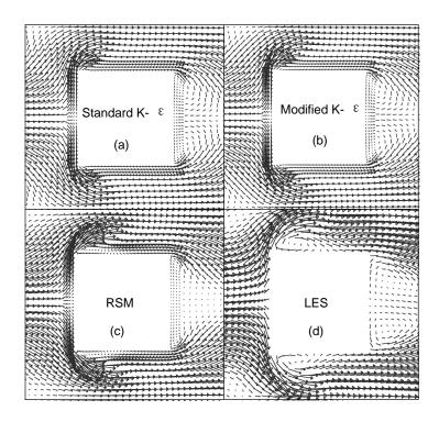
Figure 14. Mean velocity vectors in the x-y plane at z/h = 0.5. LES, medium mesh.
