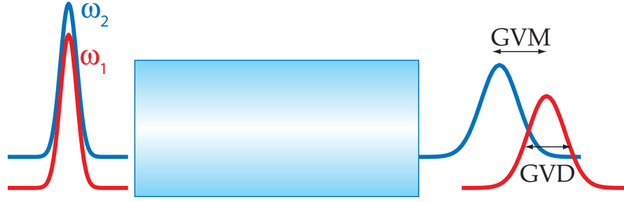
Figure 5.2: Illustration of the GVM and GVD effects on two pulses of different frequencies, \omega_1 and \omega_2 , in bulk LiNbO 3 . Given \omega_1 < \omega_2 , it follows from Fig. 5.1 that u_1 > u_2 . Whilst GVM is responsible for separating the two pulses after propagating in the material, GVD is responsible for the pulse broadening.
