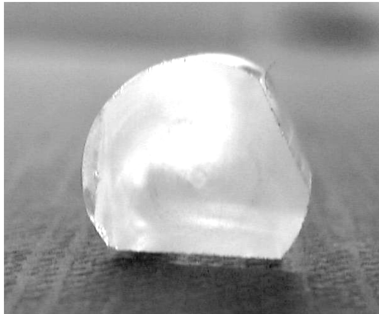
Figure 4.7. Cross-sectional view of the preform LF170 made at the ORC.
