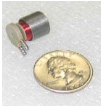
Figure 4.2: a) the miniature voice-coil actuator (H2W, NCC01-04-001) shown in comparison to a US$ quarter coin.
