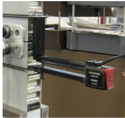
Figure 6-4: Extensometer applied to test joint
