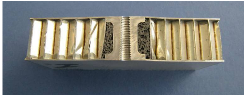
Figure 4-11: Image of a hot bonded reference sample sectioned after testing
