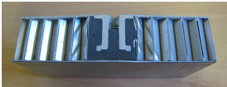
Figure 4-12: Image of a cold bonded reference sample sectioned after testing
