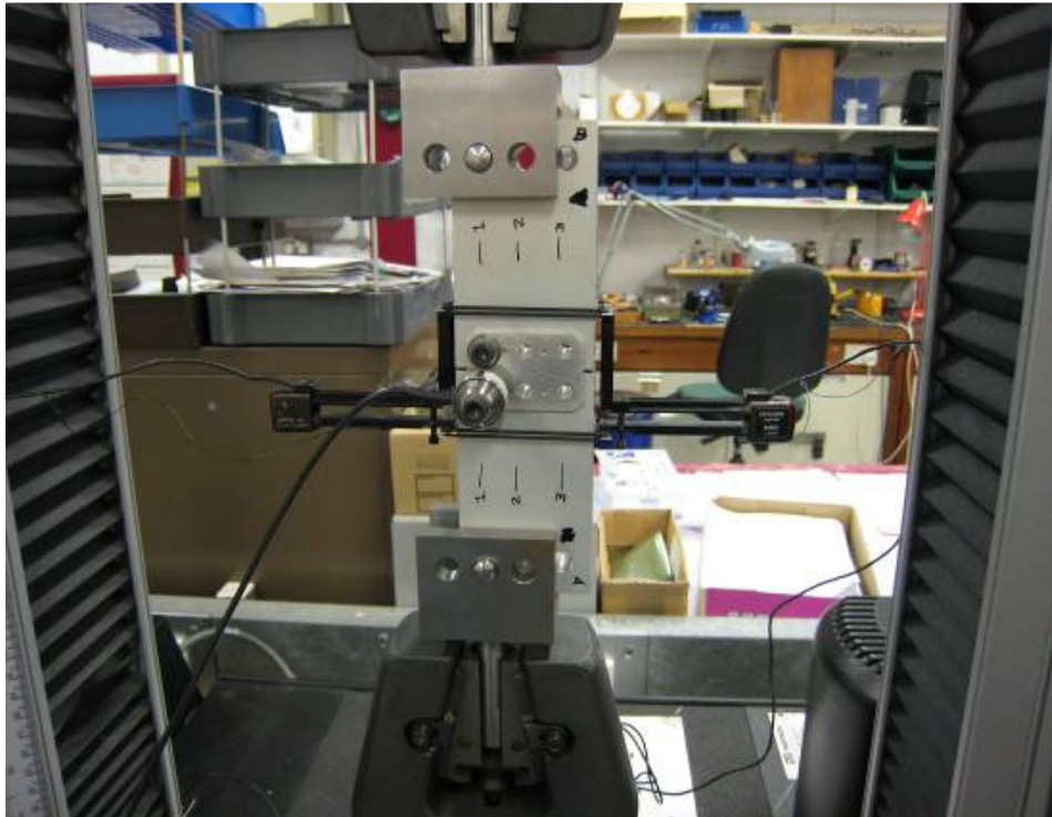
Figure 6-2: Test-joint set up in the testing machine with extensometers and load cell
