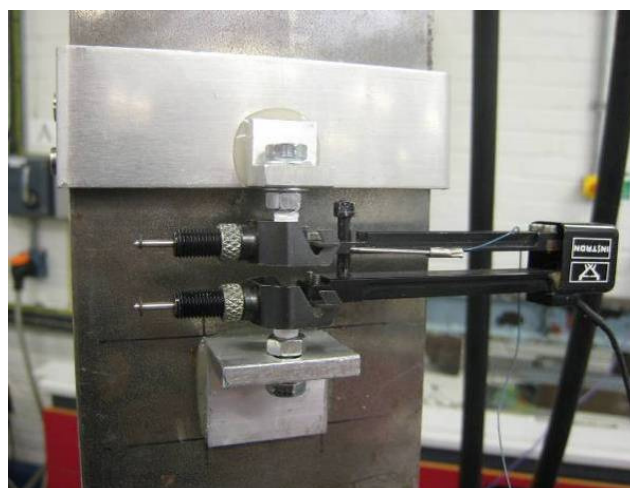
Figure 2-9: Strain gage extensometer applied to bonding plates
