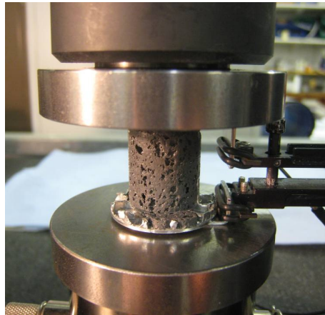
Figure 4-18: Compressive test of Redux 219/2-NA adhesive foam
