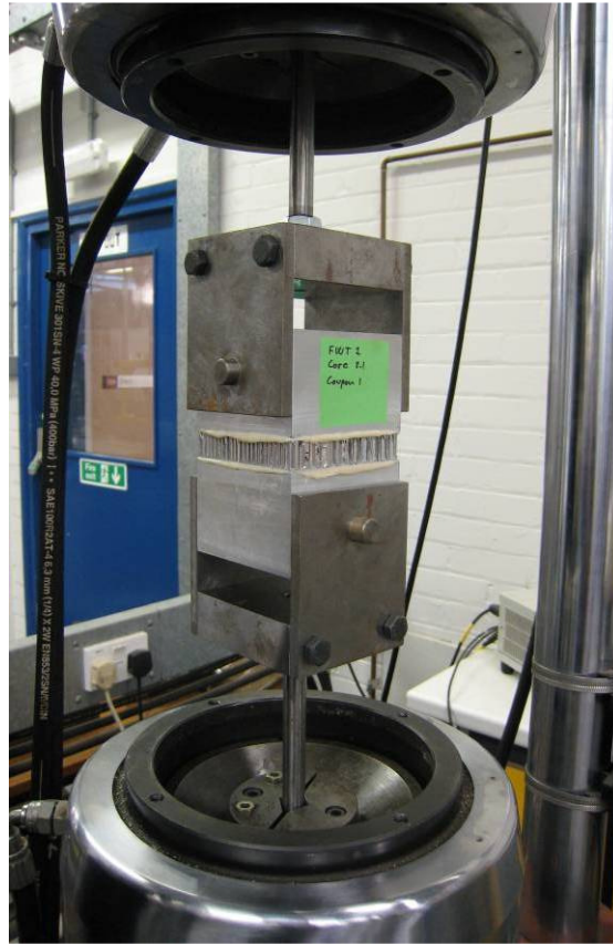
Figure 2-11: Flatwise tensile testing of a square 8.1 cored coupon
