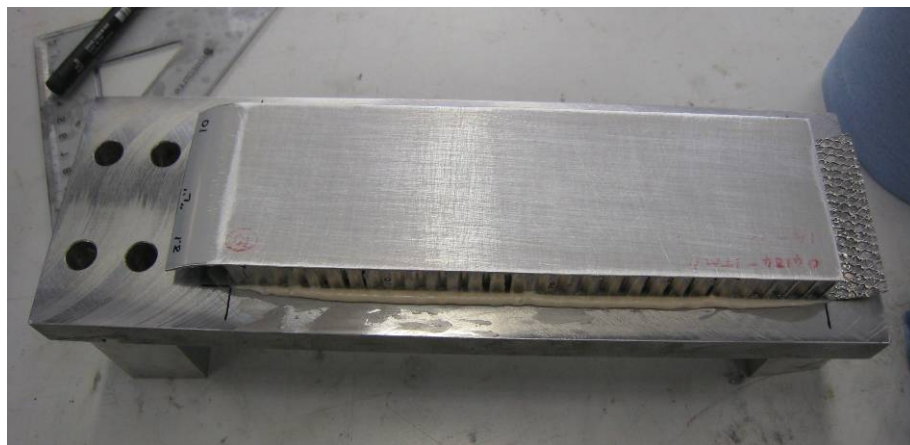
Figure 2-6: Example of one of the test coupons bonded to one of the loading plates
