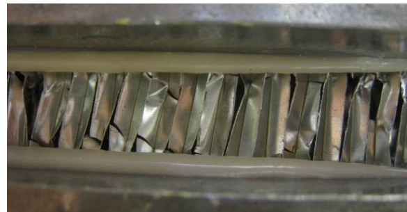
Figure 2-21: Crack development in core after fatigue testing in W direction at 35% of the static ultimate load ~718394 cycles
