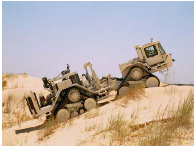
Figure 1.4 – Photograph of a source vehicle for a truck mounted vibrator. The base plate that transmits vibrations is located in the centre of the vehicle. From [113].
