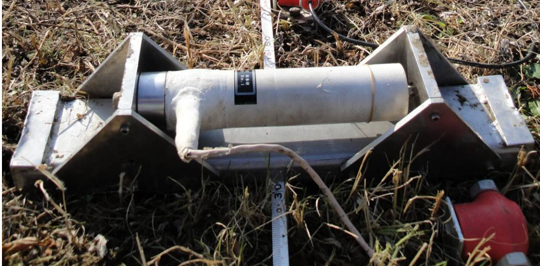
Figure 6.12 – Photograph of the seismic source used at the experimental site in Japan.
