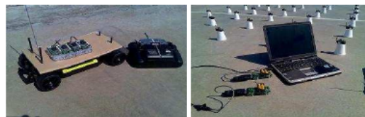
FIGURE 2.9: Dense network set up for acoustic based tracking. Reprinted from [1]
