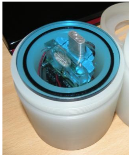
Figure 6-27 Photograph of a version 2 CT sensor system, where the conductivity sensor chip is placed vertically on the left, and temperature sensor chip is coated inside a aluminium sleeve on the right.
