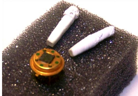
Figure-3.2: A photograph of a SensL 3035 SiPM set into a T08 can with a CsI(Tl) and a LSO crystal, both wrapped in PTFE.
