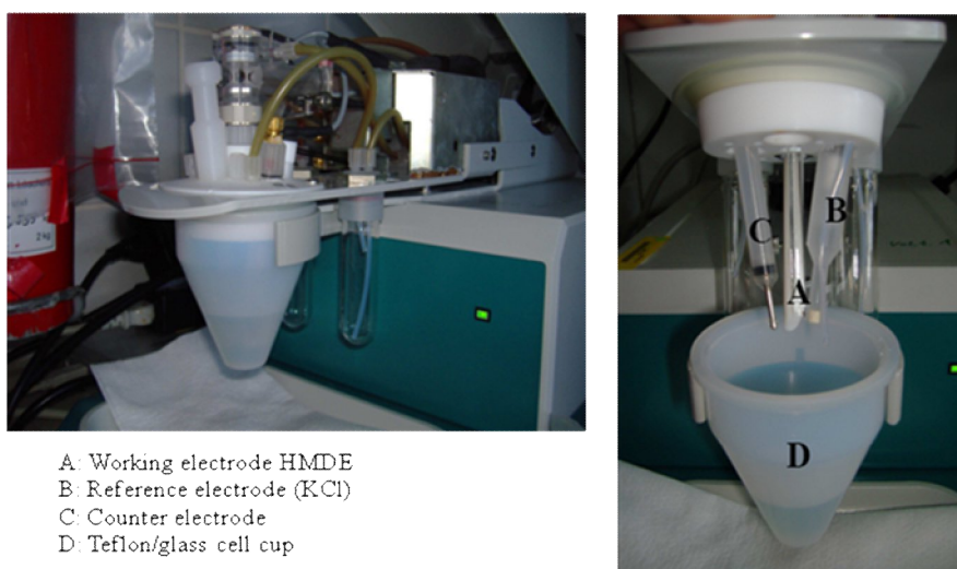
Figure 13: The voltammeter used for determination of organic Fe(III) binding ligands. Three electrodes electrochemical cell for voltammetric analysis was used; hanging mercury drop electrode (HMDE), reference electrode (KCl) and counter electrode. This instrument was set up on a Class 100 laminar airflow bench at room temperature (25°C).
