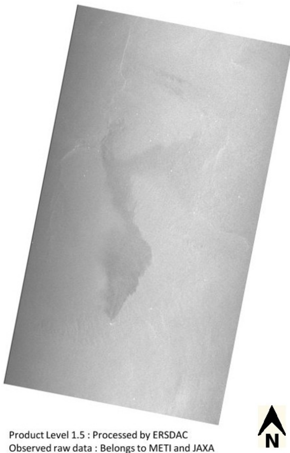
Figure A.1. The Phased Array type L-band Synthetic Aperture Radar (PALSAR) image of the Gulf of Mexico oil spill on taken on 24 th April, 2010 at 16:25 UTC. Observation mode is FBS (original resolution 100 m/pixel) at an off-nadir angle of 28.8°, path 482 and in a descending direction 1 . The use of the L-band leads to a reduction in the contrast of the spill, but shape detection is still possible.
