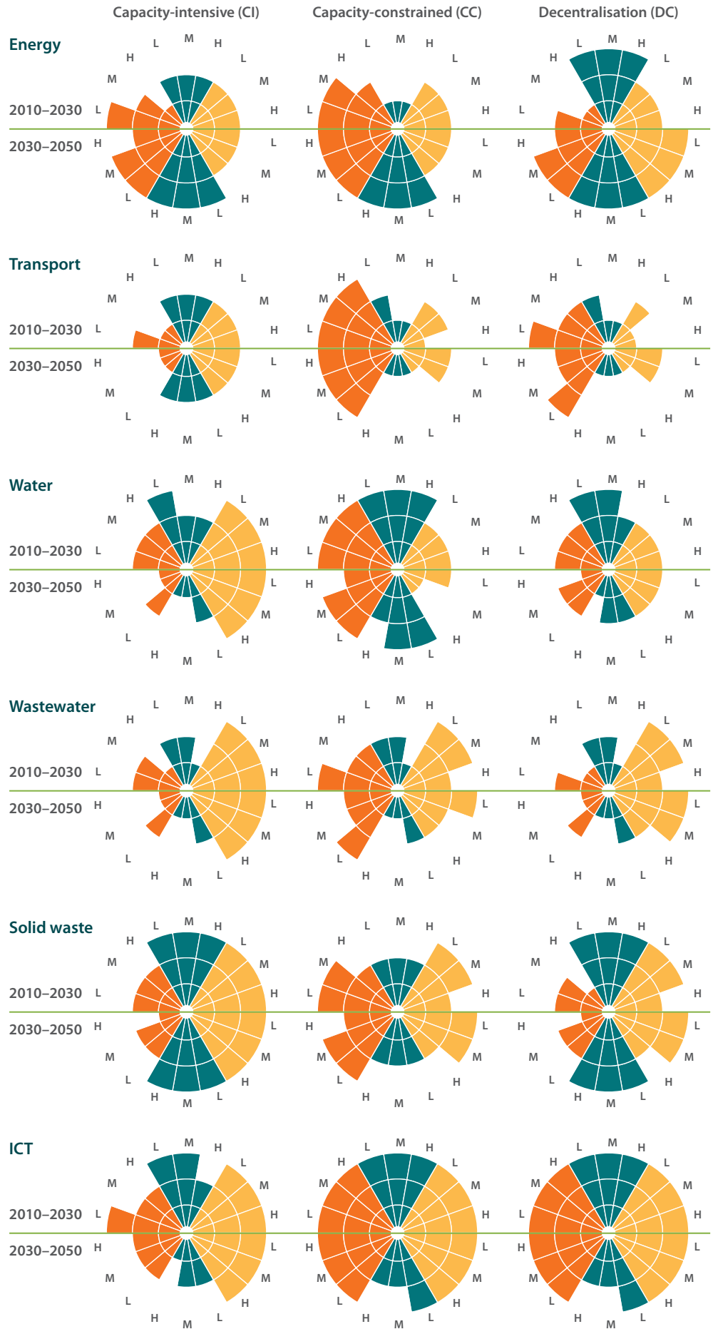
Figure 12: Summary of transition strategy performance assessment using cross-sectoral metrics of cost, emissions and security of supply. In the transport sector, the 'security of supply' metric relates to congestion.
