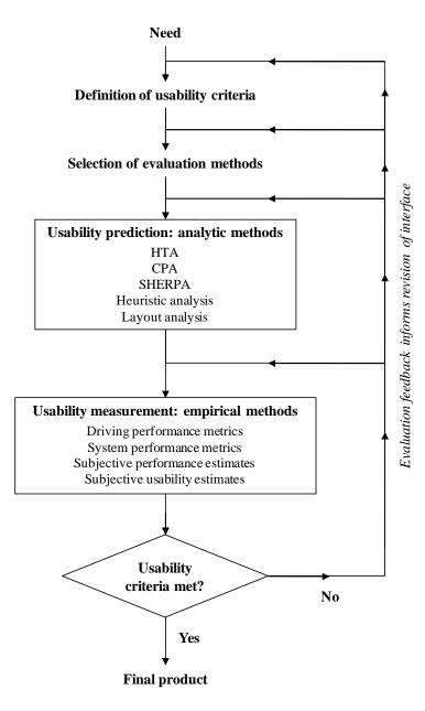
Figure 1. Framework for usability evaluation, adapted from Harvey et al. [18].
