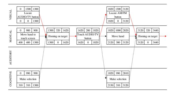
Figure 4. Excerpt of MCPA diagram for touch screen audio task, with operation timings given in ms.
