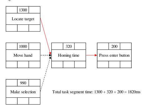
Figure 5. Excerpt from touch screen MCPA diagram to show a single target selection segment.
