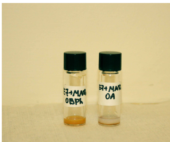
FIGURE 5.12: Photo of bottles with 1.5 wt.% concentration suspensions of OBPh (bottle on the left) and OA (bottle on the right) coated magnetite nanorods in nematic E7.
