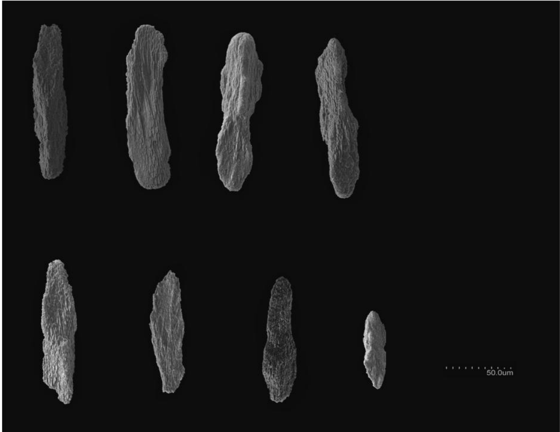
Figure 5. 29. SEM images of sclerites from the pharynx of sample Ma33 from 45°N on the Mid-Atlantic Ridge. Illustrates the presence of tapered rods within the pharynx . Scale bar = 200 μm.
