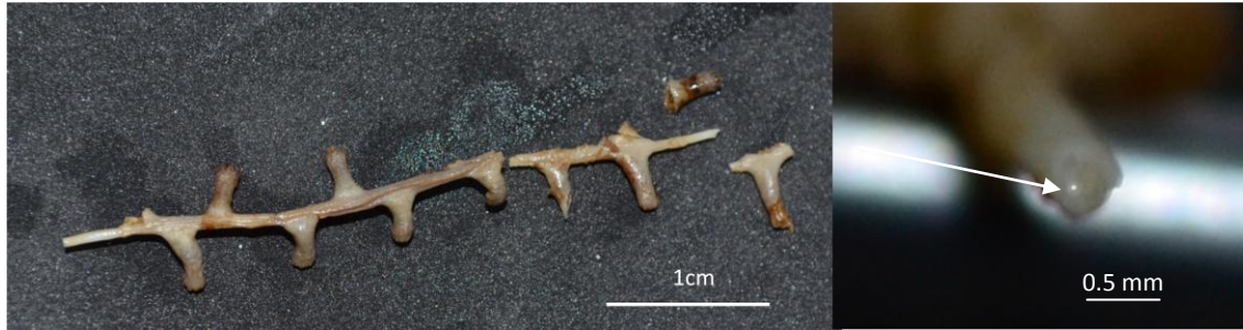
Figure 5.3. Sample Ma27 used for description collected from 45°N on the Mid-Atlantic Ridge. A) Sample specimen preserved in ethanol illustrating polyp placement and shape B) Sample core, with hollow centre illustrated by the arrow taking up less than 10 % of the diameter.
