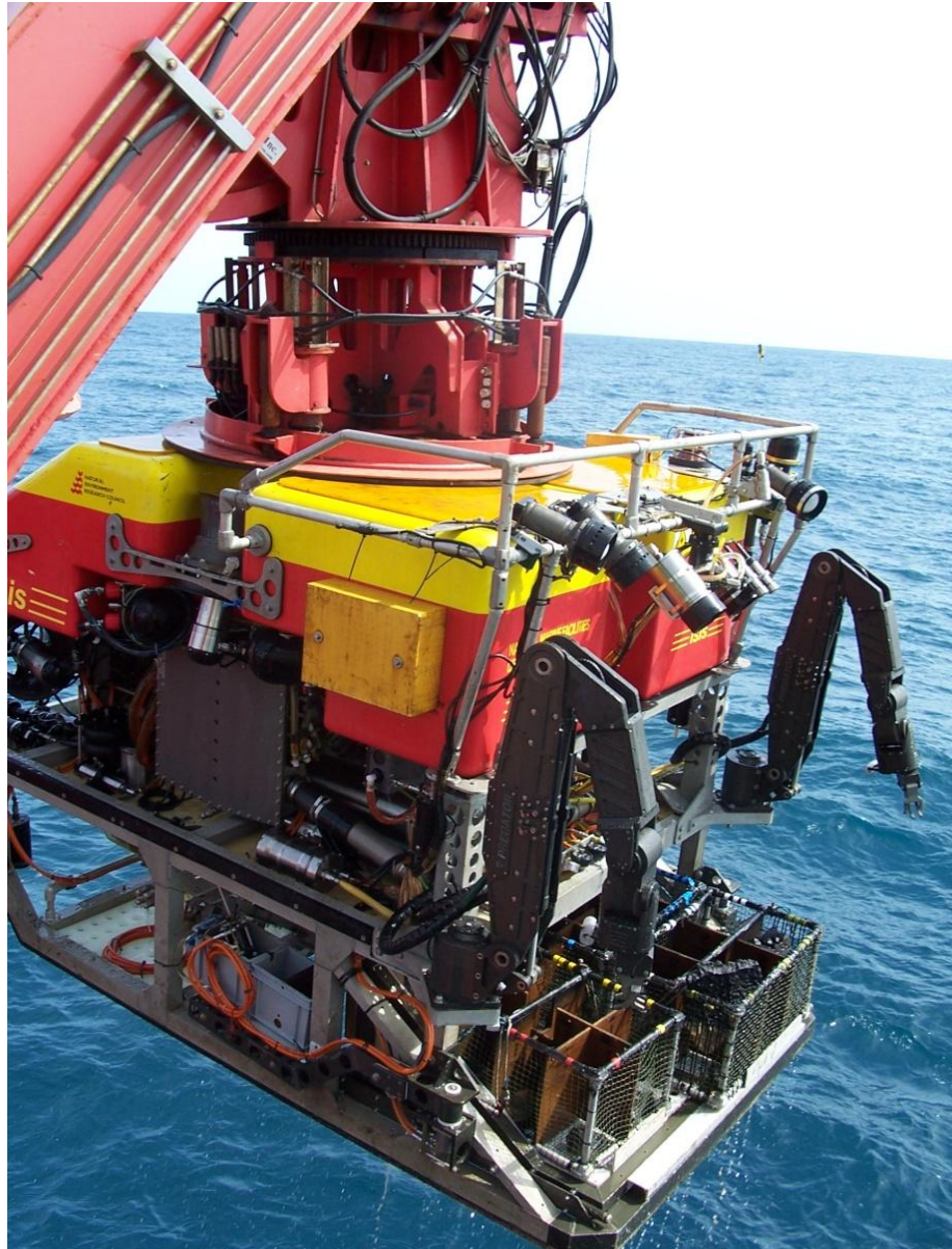
Figure 2.1. ROV Isis being deployed from the side of the RRS James Cook during JC24. It is possible to observe the pilot cameras at the front of the vehicle and rock collecting compartments.
