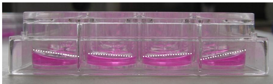
Figure B.3.6 Slanted phenolphthalein-stained Laponite hydrogels after centrifugation. Gels are flat but slanted at an angle (dotted lines) due to centrifugal force.
