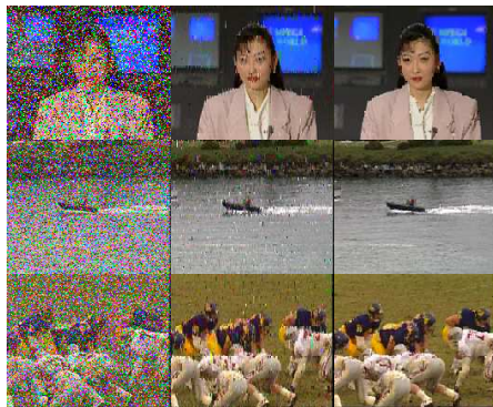
Fig. 10. Comparison of the first frames recorded at E_b/N_0 of 9.4 dB, 3.7 dB and 1.6 dB for the Akiyo, Coastguard and Football sequences, decoded by MMSE-HD, FOMM-SBSD and IHVSM. MMSE-based pixel estimation is employed.
