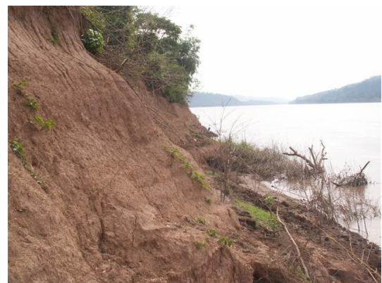
Figure 2.17. River bank stratigraphy at Ang Nyay (18°3'15.9"N 102°19'5.5"E) (photo taken in 10.2008), sand is the upper layer, clay is middle layer and mottled clay is the lower layer.
