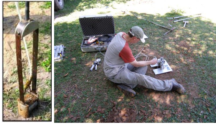
Figure 3.6. BST shear head (left) and the control system(right)
