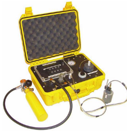
Figure 2.12. Cohesive Strength Meter (CSM) (Tolhurst et al., 1999)
