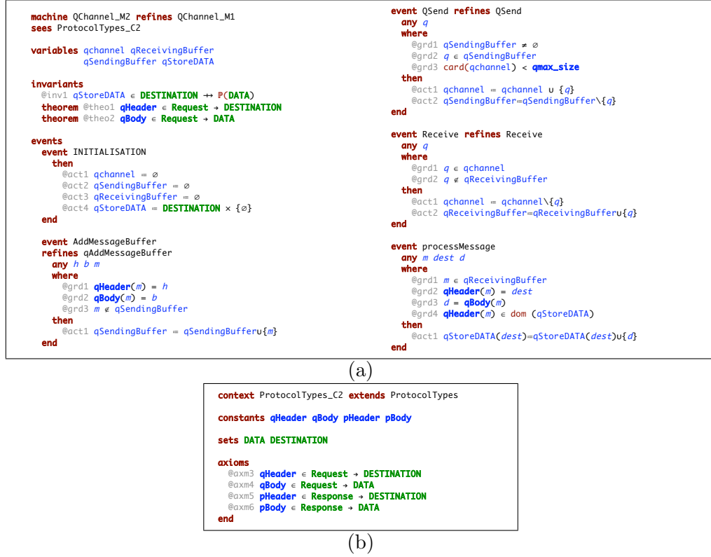
FIGURE 3.16: Expanded version of instantiated machine QChannel\_M2 (a) and context ProtocolTypes\_C2 (c)
