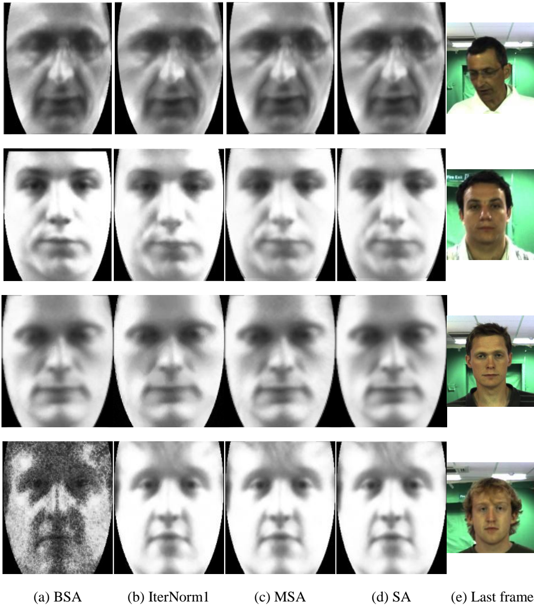
Figure 6.4: Results of the HR images and the last frame of the image sequences; HR images which are generated by (a) Bilateral Shift and Add method, (b) Iteration Norm 1 method, (c) Median Shift and Add method, and (d) Shift and Add method (e) Last frame of the image sequence
