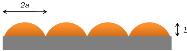
Figure 7-14. Cartoon representation of a rough surface created by spherical caps having base diameter 2a and height h . In a first order approximation the ratio between the area of the underlying surface and the surface of the caps is the same as the ratio between the surface area of a single cap and its base.
