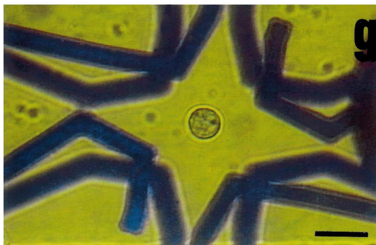
Figure 1-7. A cell trapped in an octupolar cage with broken symmetry. The electrodes are patterned on the top and bottom of a 40 \mu\text{m} deep channel, and their planes have been twisted by 20 degrees. The bar is 100 \mu\text{m} . Image taken from [64].
