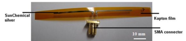
Figure 7. Inkjet printed 2.4 GHz dipole antenna on Kapton.
