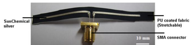
Figure 9. Inkjet printed 2.4 GHz dipole antenna on Plastibert (PU coated stretchable textile).
