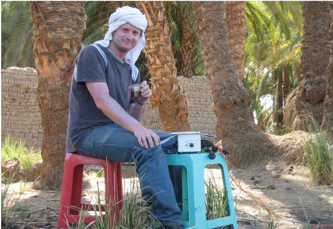
Fig. 11: Kris Strutt carrying out the ERT survey using a Geoscan Research RM15. Readings from the probe array are being taken using the instrument pictured, and recorded for later importing and computer processing (photo: Judith Bunbury).
