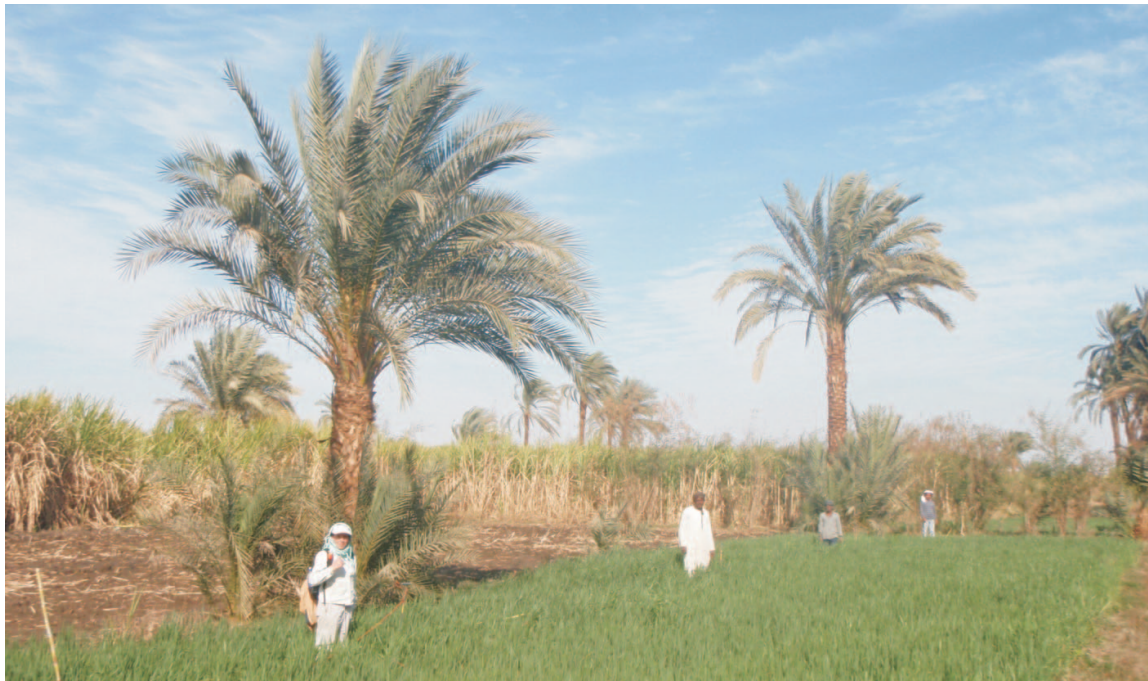
Fig. 10: Electrical Resistance Tomography (ERT) being carried out at Kom el Farahy. The workers are positioned at the current and potential probes of the Wenner configuration, with the probes in this photography set at 10m spacing (photo: Kristian Strutt).
