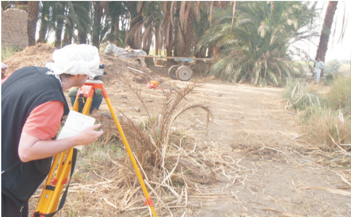
Fig. 13: Levels being taken along the profile at Kom el Farahy, allowing the topography of the site to be integrated with the ERT data (photo: Omar Farouk).
