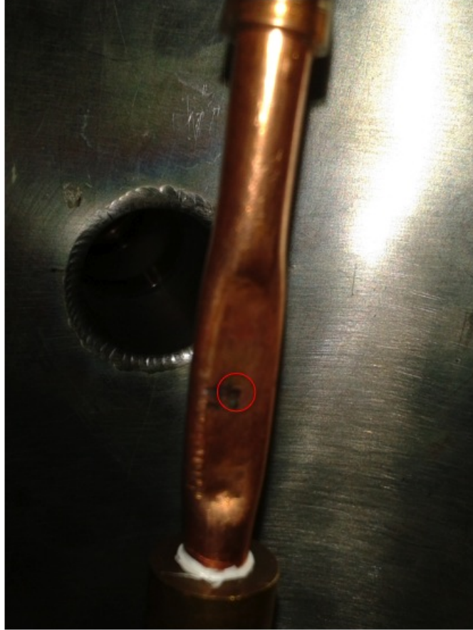
Figure 6.1: A photograph of the gas cell used in the experiments described in the next two chapters. The centre of the red circle marks the position of the 500μm input aperture
