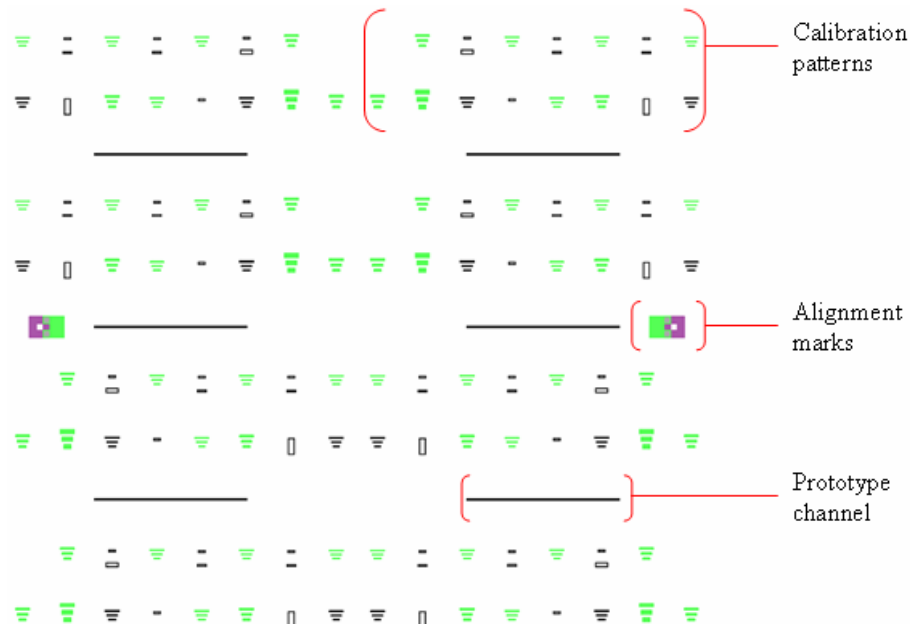
Figure 143, layout of the three layer mask design for DRIE-lag calibration patterns and prototype channels. The coloured regions indicate uncovered glass in the physical mask while the white areas indicate chrome.
