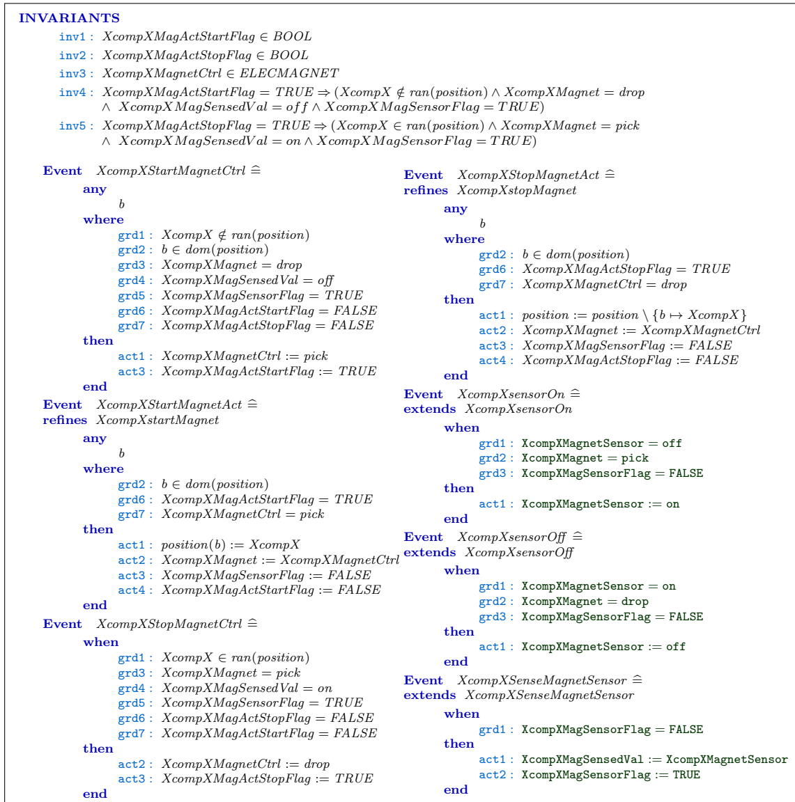
Figure 5.28: Magnet controller third refinement model
