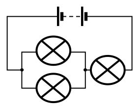
Going clockwise, draw in one colour from the battery to the first bulb, where the pd is zero. Where there is a change in potential, e.g. across a bulb, change colour and draw on the other side in a new colour. Continue back to the battery.
