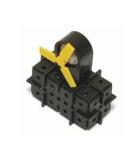
Simple motor which turns a fan to show output.
