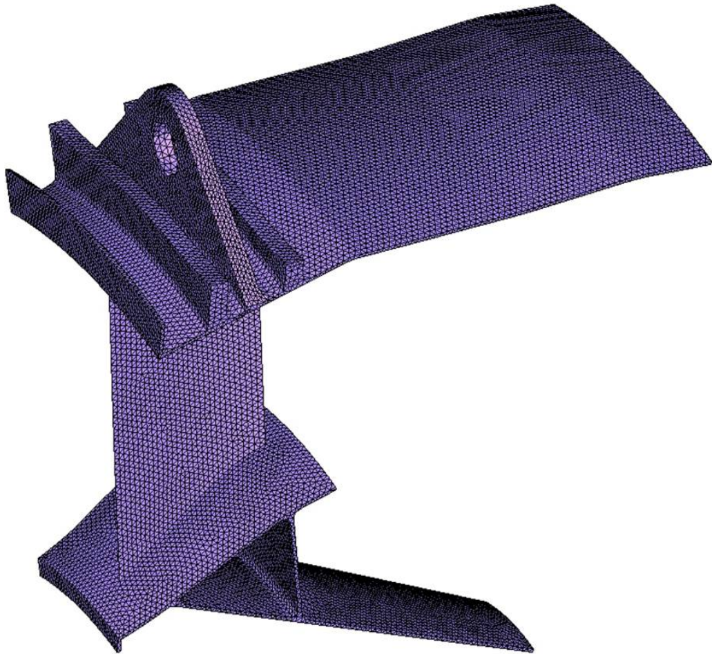
FIGURE 7.10: The solid mesh of the rear mount used to perform static analysis
