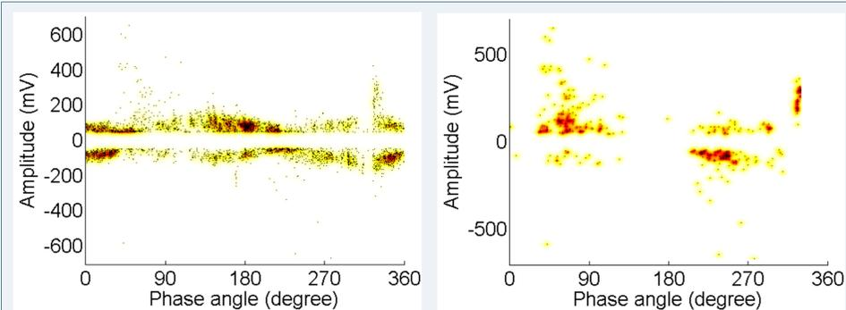
Phase resolved PD pattern of the raw data from overheating experiment
