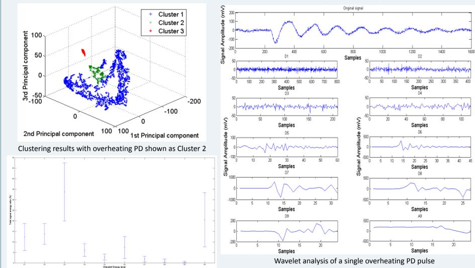
Mean and standard deviation of the WE distribution for all overheating pulses
