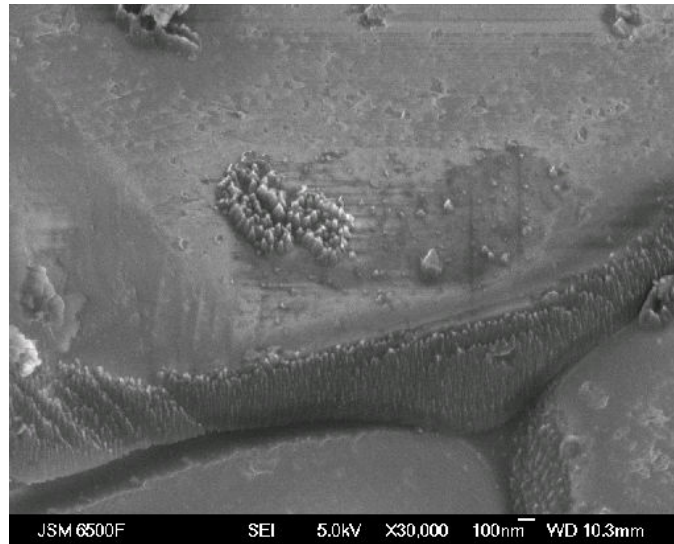
Figure 51: SEM image of remaining evaporated carbon exposed to AO
