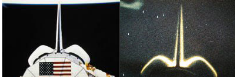
Figure 3: Solar illuminated shuttle tail-fin (left) and shuttle glow during eclipse (right). Image courtesy of NASA.
