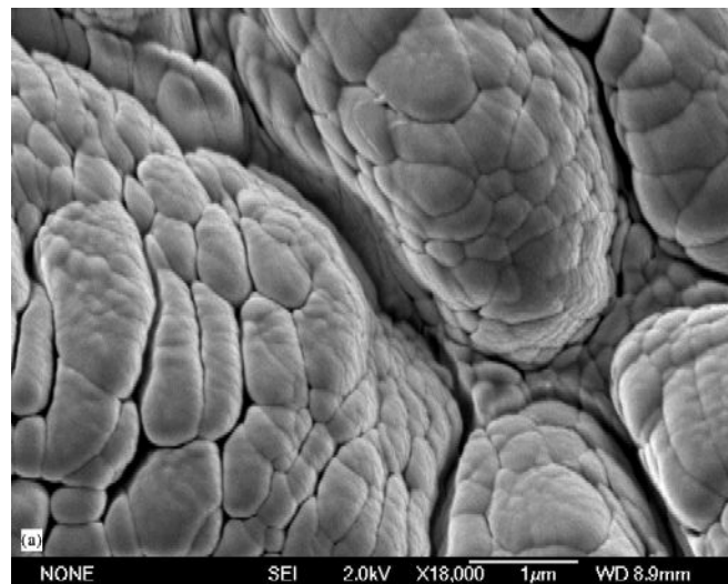
Figure 64: SEM image of sputtered film annealed to 600°C for 100 minutes
