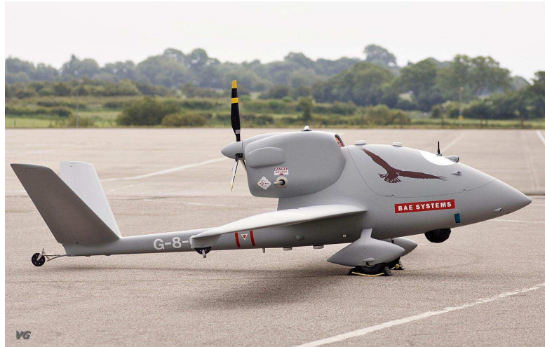
FIGURE 2.3: The BAE-Herti, a fixed wing UAV developed at BAE Systems.
