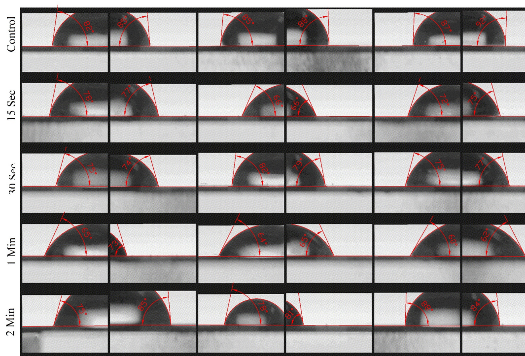
FIGURE B.9: Measurement of droplet contact angle on oxygen plasma treated Viton®
