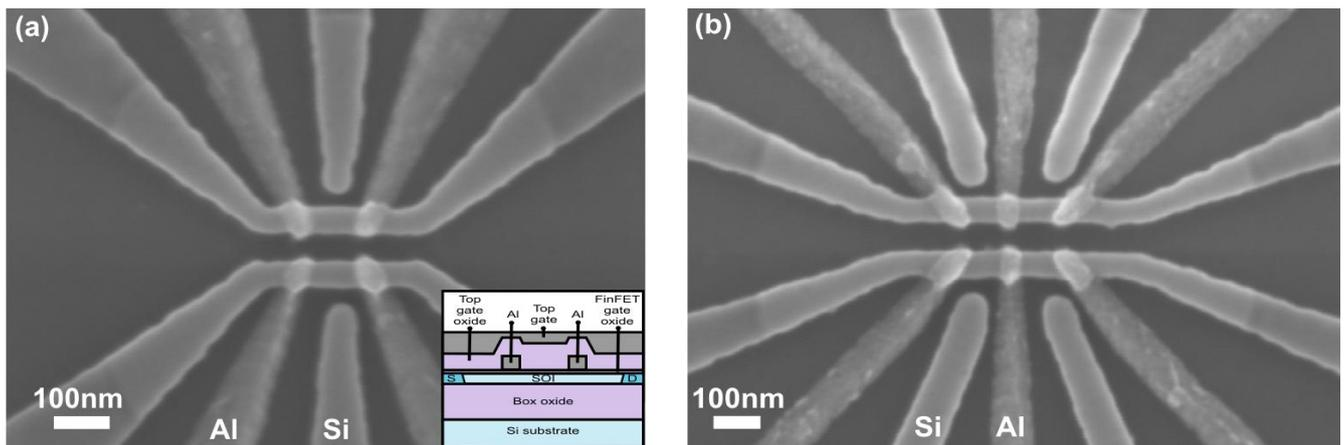
Fig. 1: SEM images of the Al FinFET turnstile and electrometer, (a) single QD turnstile and electrometer, inset figure shows a cross section schematic of the structure, (b) double QDs turnstile and electrometer.
