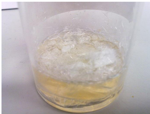
Figure 3.37 - Crystal formation on the surface of a P(MMA-co-PEGM) gel. These crystals of triethylamine formed upon leaving the gel in storage for several weeks.
