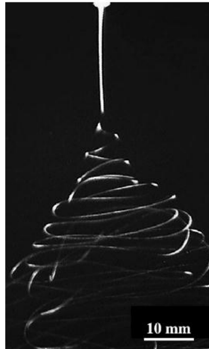
Figure 3.3 - Image of an electrospinning jet showing bending instabilities. Reprinted from Han et al. , Polymer , 2007, 48, 6064-6076, Copyright (2007) with permission from Elsevier.
