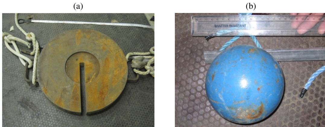
Figure 3.14. Two of the targets used from the tests with (a) a miscellaneous steel weight of diameter 0.46 m and thickness 0.05 m and (b) spherical weight of diameter of 0.12 m.
