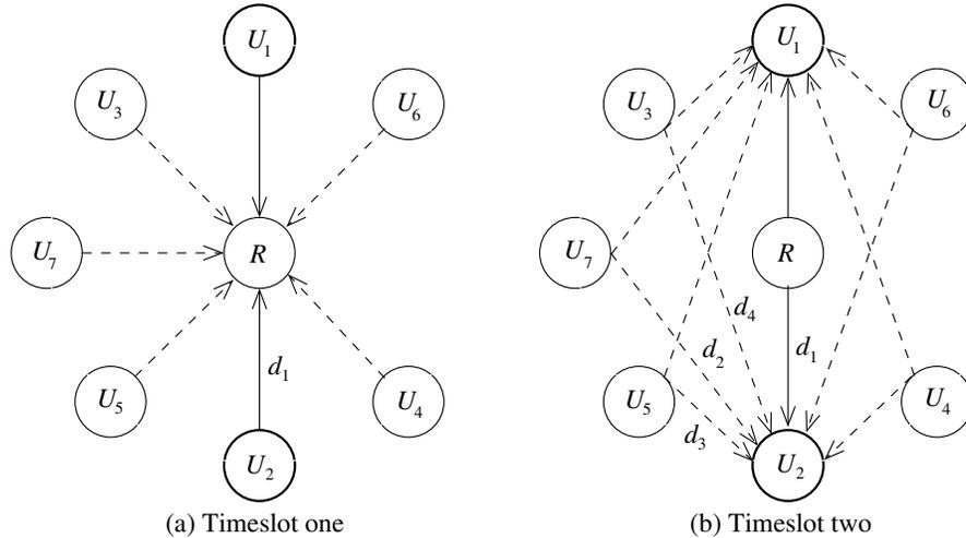
Figure 1: Two-way relaying transmission for users  $U_1$  and  $U_2$ , in the presence of five interfering users, with the aid of a relay node, in the **circular model (m1)**. The corresponding normalized distances (and geometrical gains) are given by:  $d_1 = 0.5$  ( $G_1 = 4$ ),  $d_2 = 0.7071$  ( $G_2 = 2$ ),  $d_3 = 0.3827$  ( $G_3 = 6.8283$ ) and  $d_4 = 0.9239$  ( $G_4 = 1.1716$ ).
