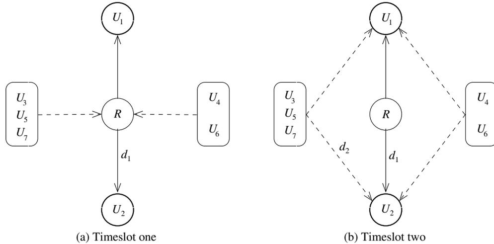
Figure 2: Two-way relaying transmission for users  $U_1$  and  $U_2$ , in the presence of five interfering users, with the aid of a relay node, in the **triangular model (m2)**. The corresponding normalized distances (and geometrical gains) are given by:  $d_1 = 0.5$  ( $G_1 = 4$ ) and  $d_2 = 0.7071$  ( $G_2 = 2$ ).
