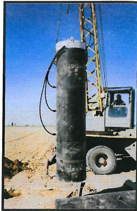
Plate 3.2 Lysimeter Prior to Field Insertion Showing Tensiometer Connections
