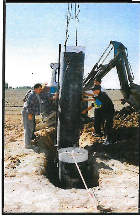
Plate 3.3 Field Insertion of the Lysimeters
