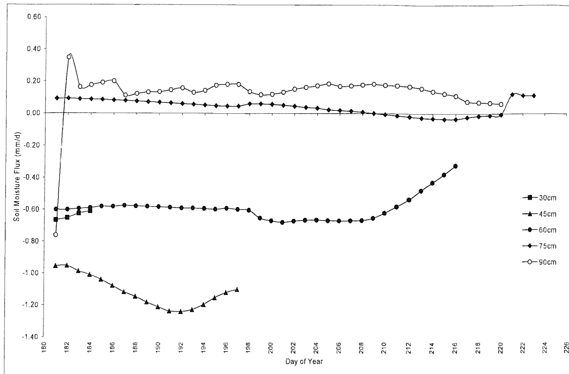
Figure 5.10 Daily Soil Moisture Change Calculated Using Darcy's Law, Field B1
