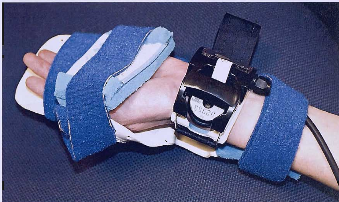
Figure 13. A heat-moulded plastic wrist splint to minimise the influence of movement on radial arterial pressure measurements. Although the Vasotrac is considerably more motion-tolerant than other blood pressure tonometers, movement of the hand and wrist frequently results in a failure to reliably detect blood pressure waveforms. The self-calibration sweep of the sensor assembly takes some time to complete and therefore, unlike other tonometers, a missed recording is costly in terms of time between measurements. Children, in particular, move during stress. Therefore, there was a requirement for a mechanism to minimise this problem. I designed a wrist splint using heat-mouldable plastic, memory foam padding and soft Velcro straps to comfortably hold the subjects' hands still during the experiment. A channel at the back of the splint prevented it from impinging on the strap of the Vasotrac. The thumb was separately restrained and finger straps and a palm block held the fingers and hand in place.
