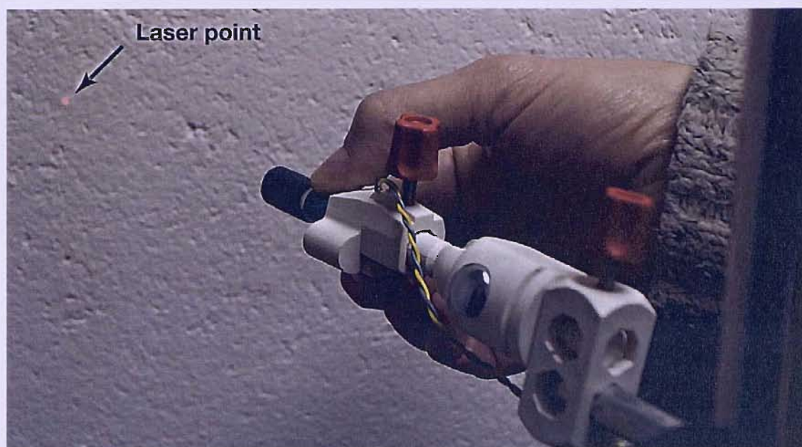
Figure 21. Demonstration of the laser-levelling device in use. In practice, the device was used on a level hard floor (laid with self-levelling compound). The subject's height was measured whilst they stood on a stadiometer having been positioned appropriately for height measurement with their head in the Frankfurt plane and their neck supported by an assistant. With the subject still in this position, the height of the electrodes which were fixed according to anatomical landmarks was determined by casting the laser point on the landmarks and then onto the ruler of the stadiometer. A computer calculated the positions of the other electrodes and these positions were 'read off' the stadiometer before the beam was cast onto the skin and marked with a skin marker.
