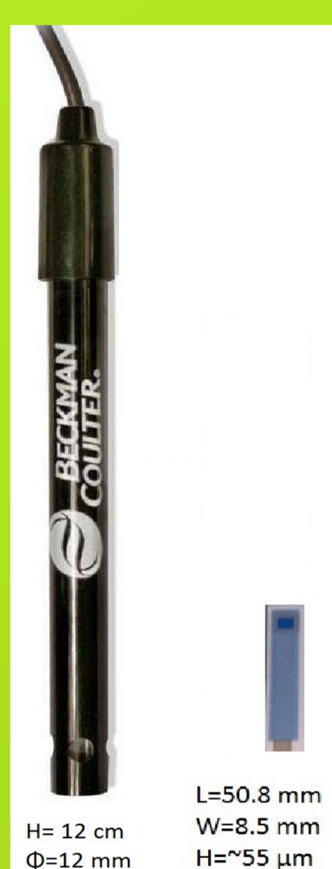
Figure 2: A commercial silver/silver chloride (Ag/AgCl) reference electrode (left), Thick-Film electrode (right).
