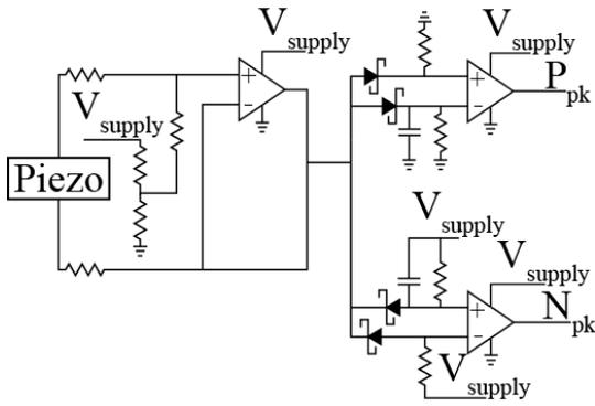
Figure 6: Low power peak detection circuit [7].
