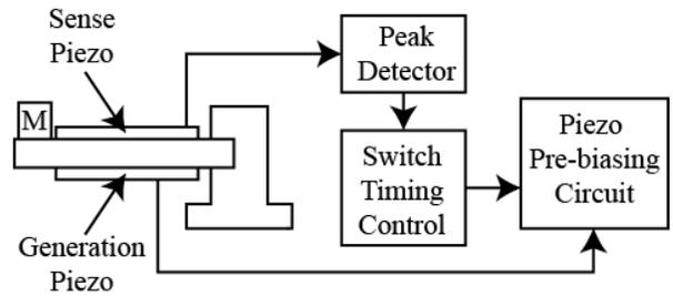
Figure 4: Multilayer piezo connected to SSPB circuit implementation.
