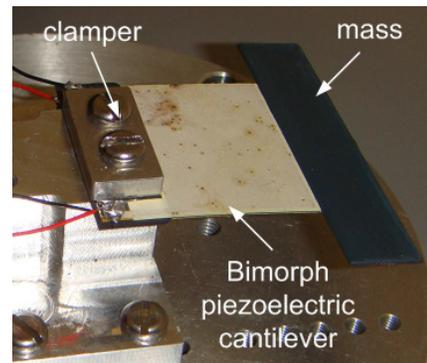
Figure 5: Photo of the multilayer piezo energy harvester.
