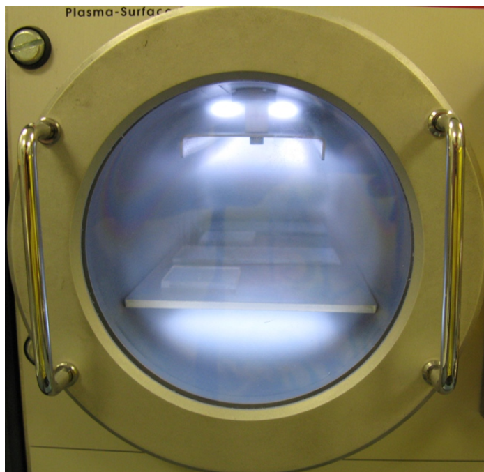
Figure 4.5: Glass and PDMS samples undergoing oxygen plasma exposure.
