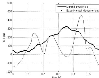
Fig. 7. Experimental R-T measured during one kick cycle for a tow speed of  $2.23 \text{ ms}^{-1}$  and a kicking frequency of 1.7 Hz. The predicted thrust from EBT is deducted from the mean predicted drag to produce a predicted R-T
