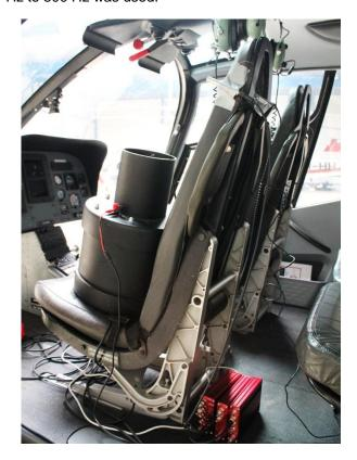
Figure 2 – Measurement setup during transfer path scanning measurements
