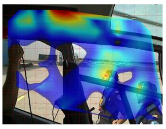
Figure 5 – Pressure contribution mapping between 50 Hz and 100 Hz with a 10 dB dynamic range
