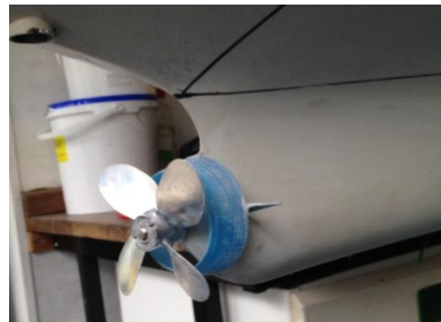
Duct (based on Mewis Duct)
