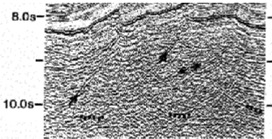
Figure 2. Migrated multichannel seismic reflection profile (from Charles Darwin cruise 28-CD28; Bull and Scrutton, 1990, 1992). Location of the line is displayed in Fig. 1. Reverse faults cutting through the crust are indicated by arrows and possible Moho reflections are highlighted by dots. Vertical scale is in seconds, two-way travel time.
