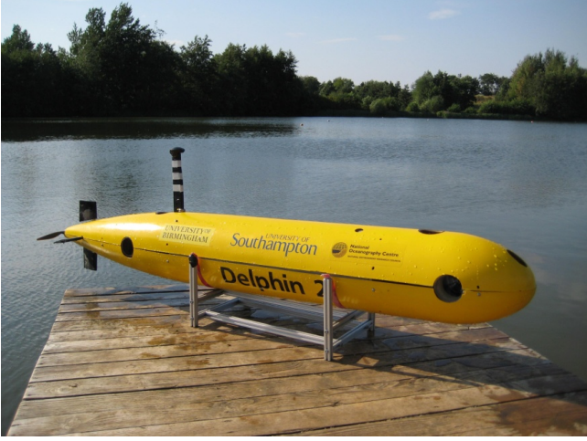
Fig. 1. Delphin2 AUV: Over-actuated hover capable AUV stability. The thrusters are the dominant actuator set when operating between minus 0.3 \text{ ms}^{-1} to plus 0.5 \text{ ms}^{-1} forward speed.
