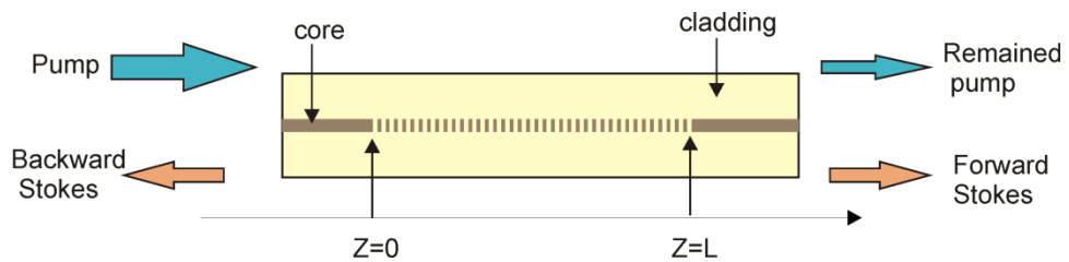
Fig. 3-2 Schematic diagram of the Raman DFB fibre laser in a uniform FBG.
