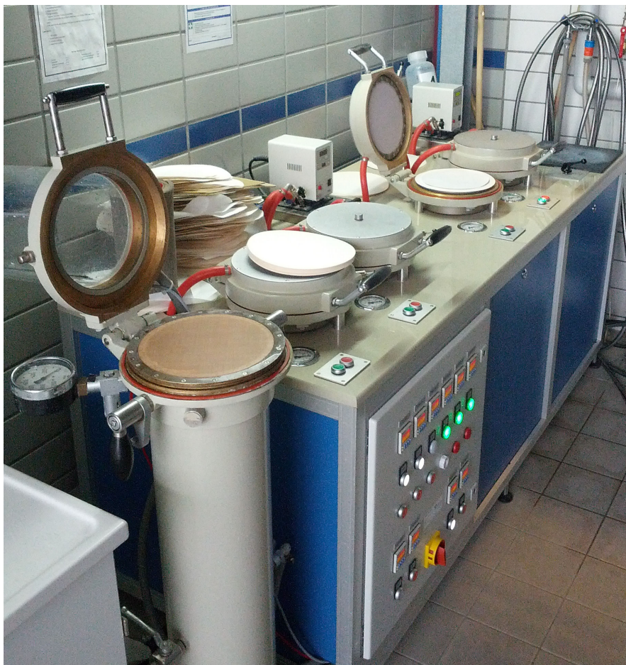
FIGURE 7.6: Rapid-Köthen Sheet Former by FRANK Prüfgeräte GmbH.
