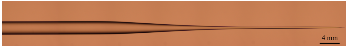
Figure 4.4: Image of a fiber tip with diameter of 50 nm used to collect signals from the CdSe/CdS nanocrystal/silica microsphere hybrid resonators.
